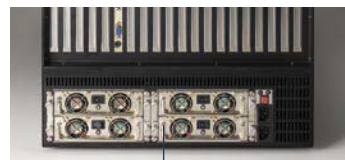
Hot-swap redundant power supply
